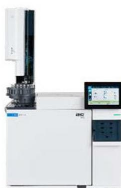
PAC Powered by AC offers a guaranteed and turn-key analyzer, as part of its analyzer portfolio for petrochemical industry, that meets all the requirements as listed in ASTM D7504.
