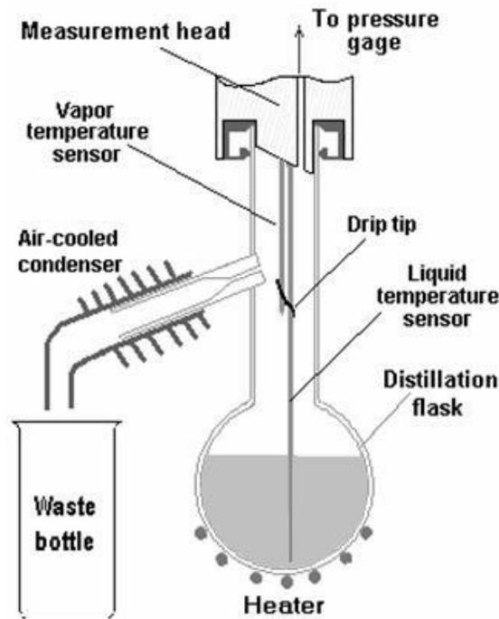
Illustration 2 – Schematic of Microdistillation flask
