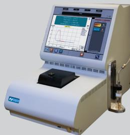
There is little training needed, as an operator only needs to fill up a vial of sample and press a button to start. A 48-place autosampler is optional if more throughput and automation are desired. No solvent is needed as the next sample is used to flush out the previous one.
