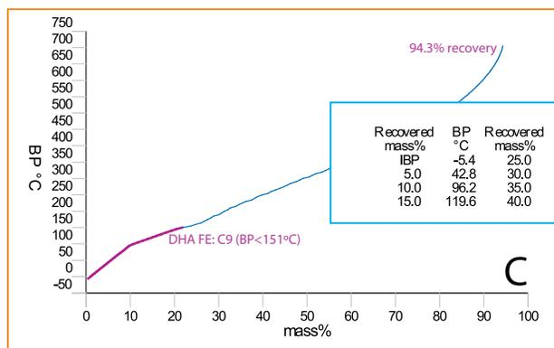
Boiling Point Mass Distribution for C, N and S for a Crude Oil Sample
