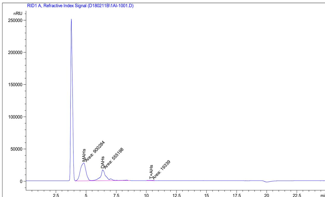
Figure 2: Chromatogram Reference Gasoil
