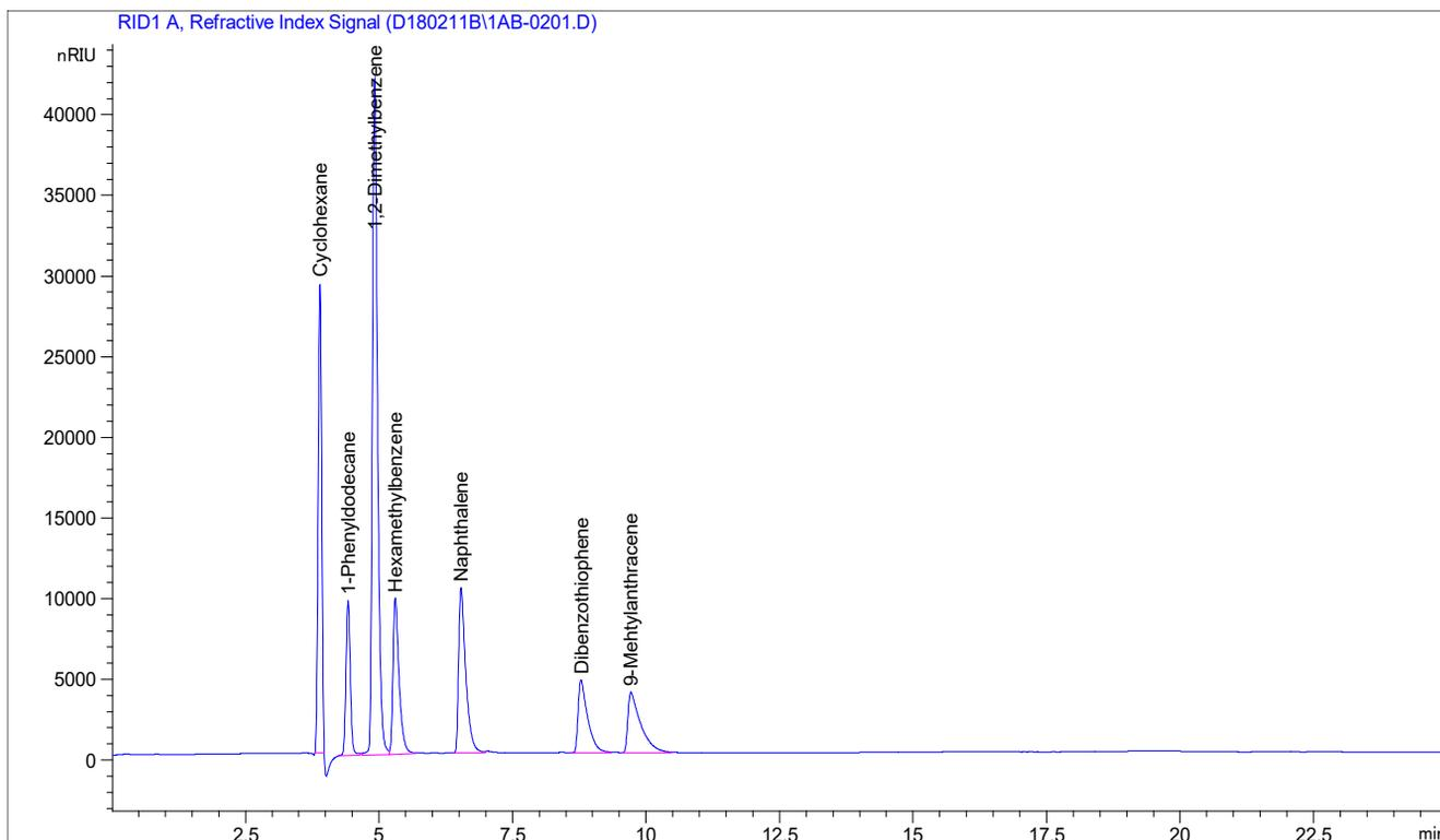
Figure 3, Chromatogram EN 12916 System Calibration Standard (SCS 1)
