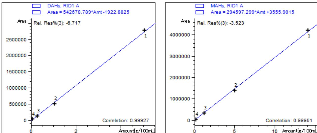
Figure 4: linearity plots for MAH & DAH
