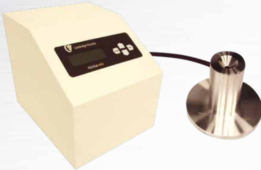
The Cambridge Viscosity ViscoLab 4000 Small Sample Viscometer utilizes oscillating piston technology and an embedded PT100 temperature sensor to provide exceptionally accurate viscosity and temperature readings.
