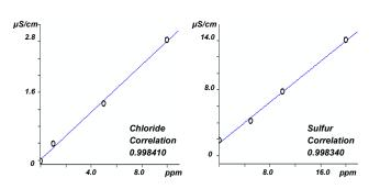
A four level calibration was made using certified sulfur (dimethyl sulfide) in biodiesel standards spiked with trichloroacetic acid for source of chloride. CIC calibration is performed through entire sample flow path
