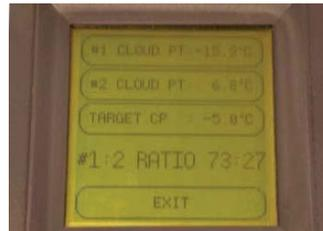
By pressing the “blends” button on the T30’s screen, you can estimate the blend ratio necessary to achieve a target cloud point given the cloud points of two starting components. Perfect for diesel and biodiesel blending.
