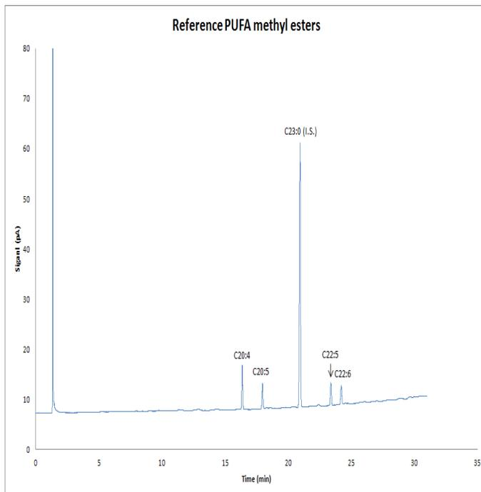
Figure 2: Chromatogram of Reference sample, containing the four predominant PUFA methyl esters and Internal standard (C23:0)
