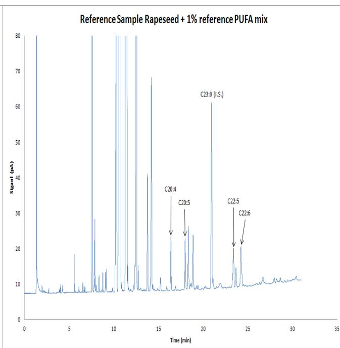
Figure 5: Reference biodiesel sample (rapeseed source) + 1 % added Reference PUFA mixture (0,25 % each PUFA methyl ester).
