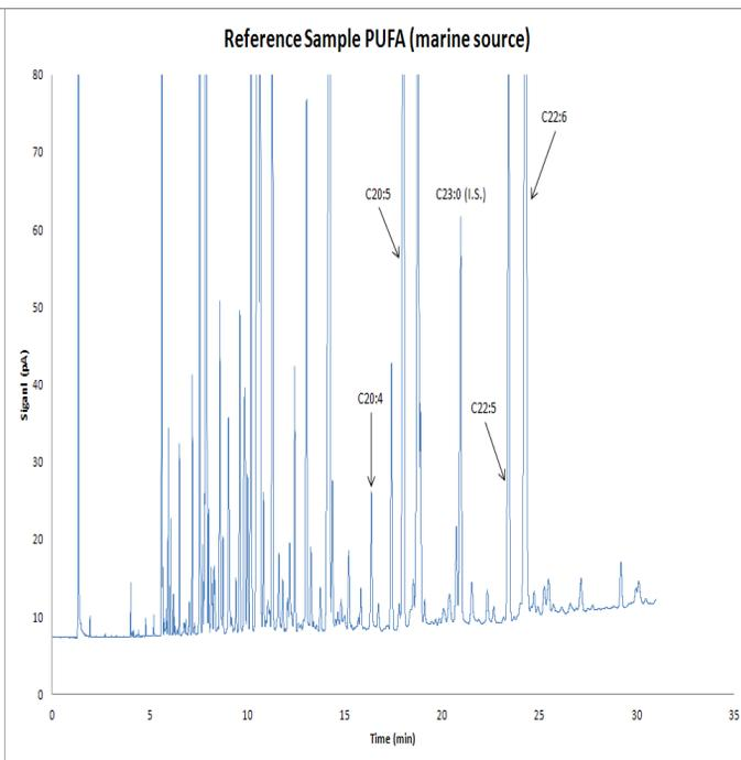
Figure 3: Reference sample PUFA (marine source). Sample contains approximately 16.0 % total PUFA methyl esters.
